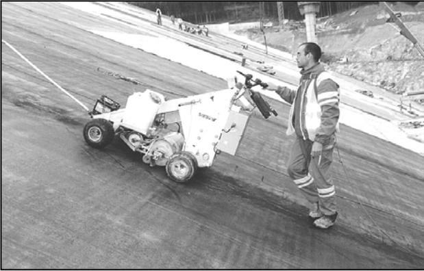
Figure 8. Ultrasonic control by CAC94 equipment
